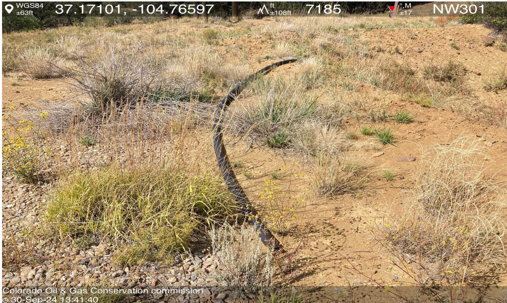
PHOTO 6: UNUSED EQUIPMENT (2" POLY PIPE). REMOVE UNUSED EQUIPMENT PER RULE 606. CA DATE 10/30/2024.
