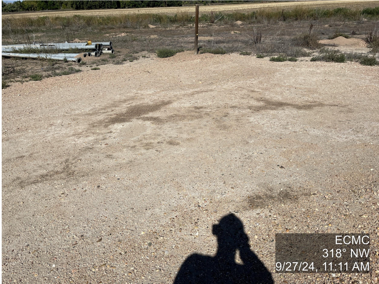
Photo 6. The photo was taken at the tank battery facility facing Northwest. The photo illustrates stained soil on the production pad.
