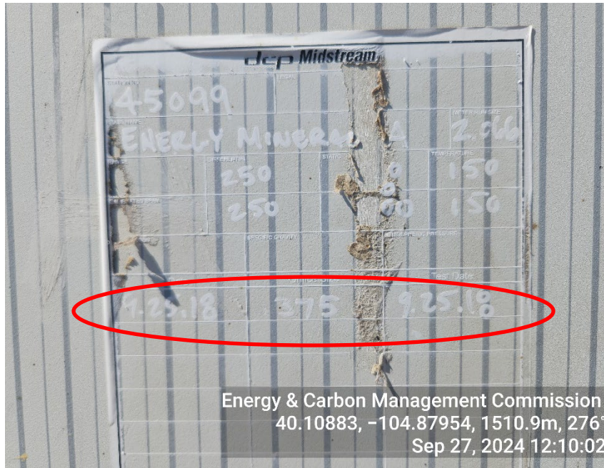
Photo 9: Meter not annually calibrated
