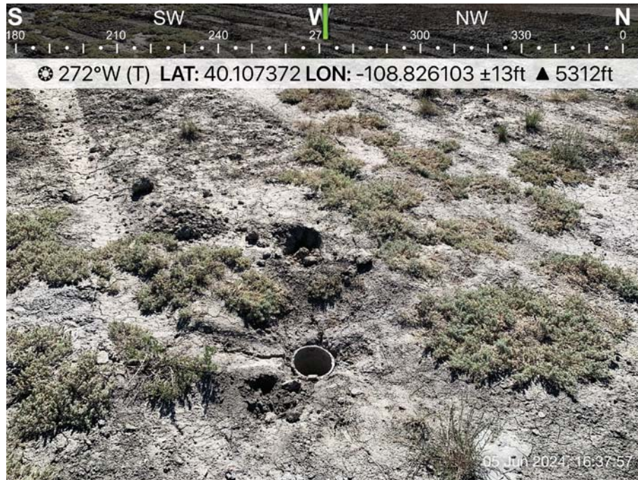
Photo 5: Silver King Pan Am Hayes #5-27 (OWP) P&A wellhead, no methane detected, view west.
