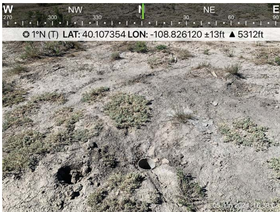
Photo 2: Silver King Pan Am Hayes #5-27 (OWP) P&A wellhead, no methane detected, view north.
