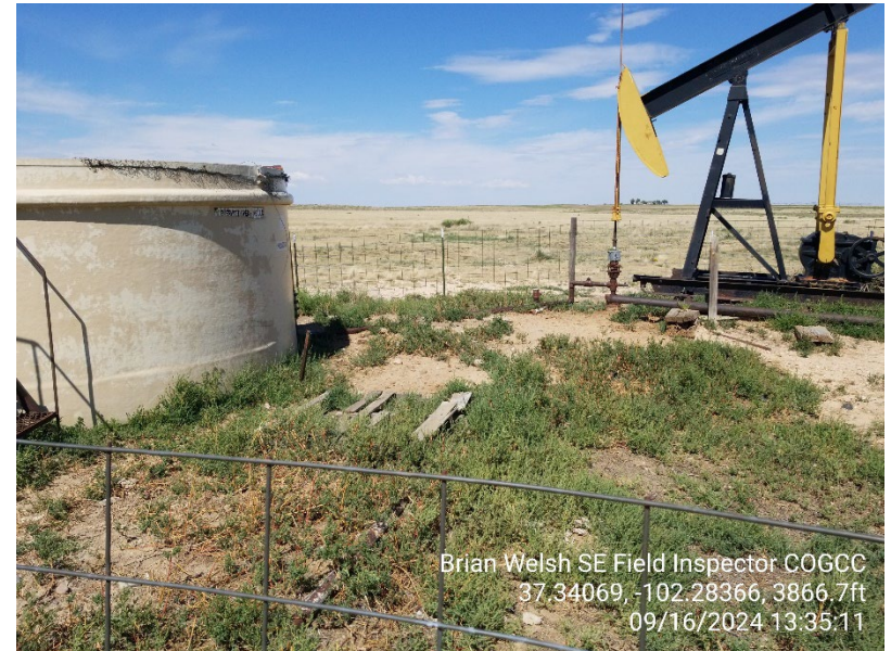
2. Water tank needs berms installed
