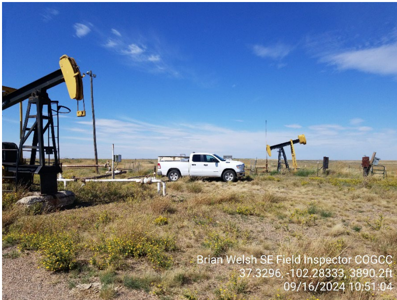
1. Location photo showing pumping unit being stored on location and gathering line on east side of wellhead
