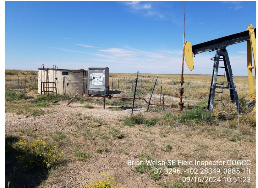
2. Pumping unit, water tank and meter run
