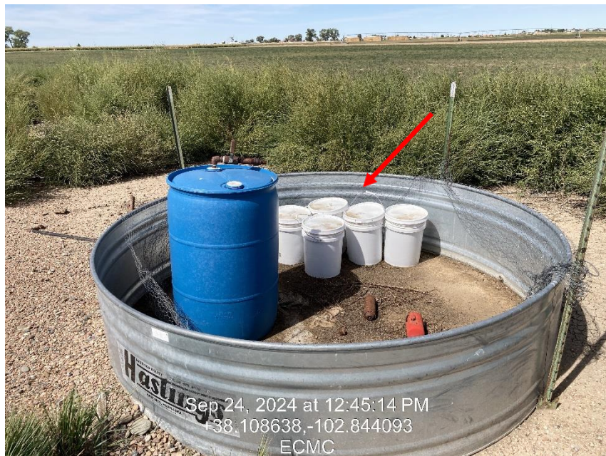
Photo 7 – Secondary Containment with impacted soils stored in 5 gallon buckets
