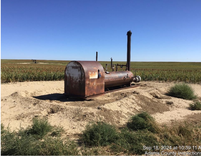
Photo #5 Separator and weeds with in set back.
