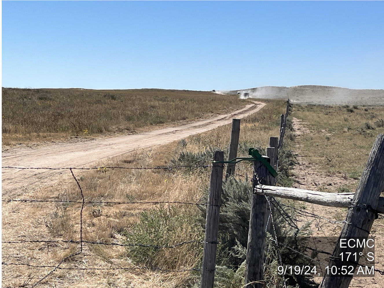
Photo 11. The photo was taken along the access road to the well location facing South. The photo illustrates wind erosion in the form of dust along the access road caused by truck traffic.
