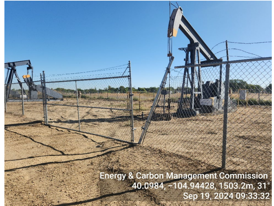
Photo 14: Fencing in disrepair
