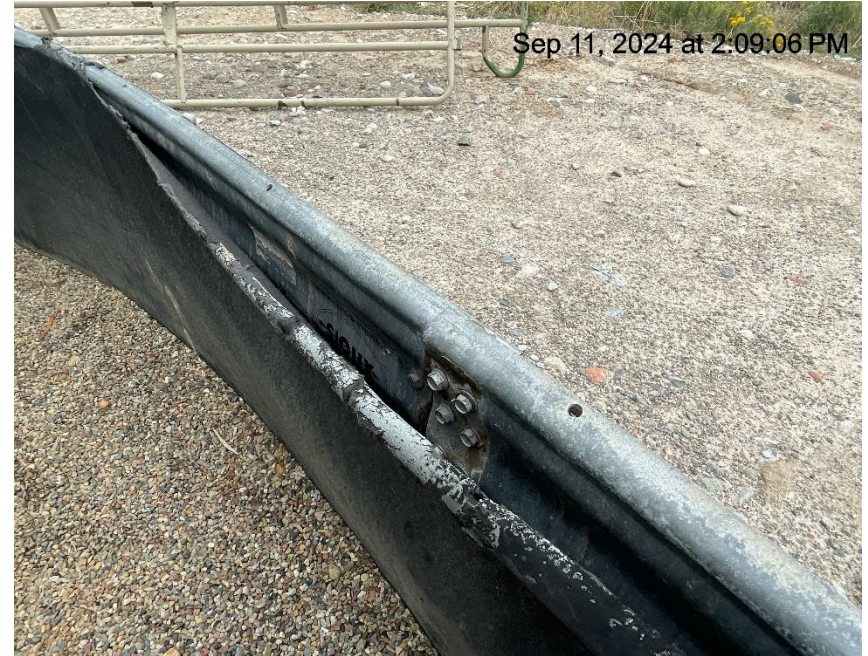
Photo # 9834 Secondary containment liner showing some signs of damage near top of containment ring
