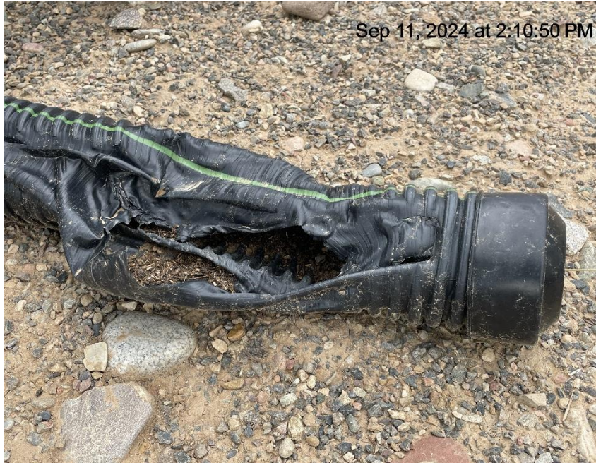
Photo # 9835 Flowline heating insulation damaged/open to entry by wildlife/wildlife hazard
