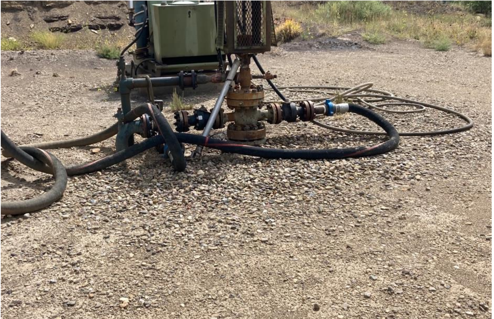
PHOTO 2: THE LEAK AT THE WELL HEAD HAS BEEN REPAIRED AND ANY STAINED SOIL HAS BEEN REMOVED.
