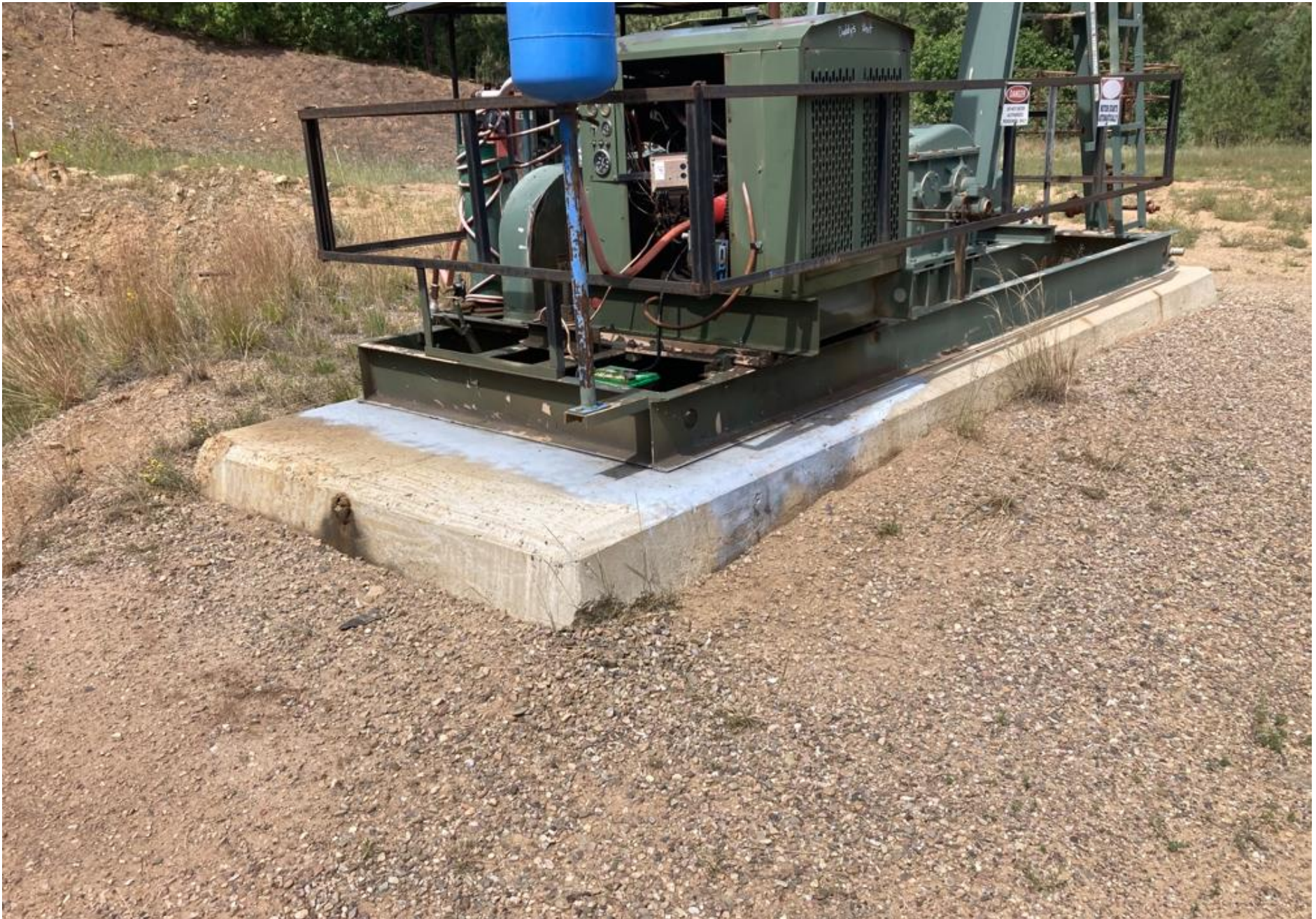
PHOTO 1: MAINTENANCE HAS BEEN PERFORMED ON ALL OPERATING EQUIPMENT. THE SOIL STAIN HAS BEEN CLEANED UP AND REMOVED FROM LOCATION, THE CONCRETE RISER HAS BEEN PAINTED TO REMOVE THE STAIN.
