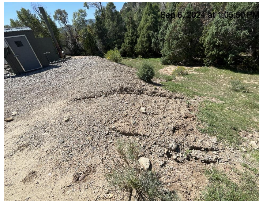
Photo # 8751 Erosion on slope & transport of sediment off location & into a vegetated area (near Summit Midstream meter house)
