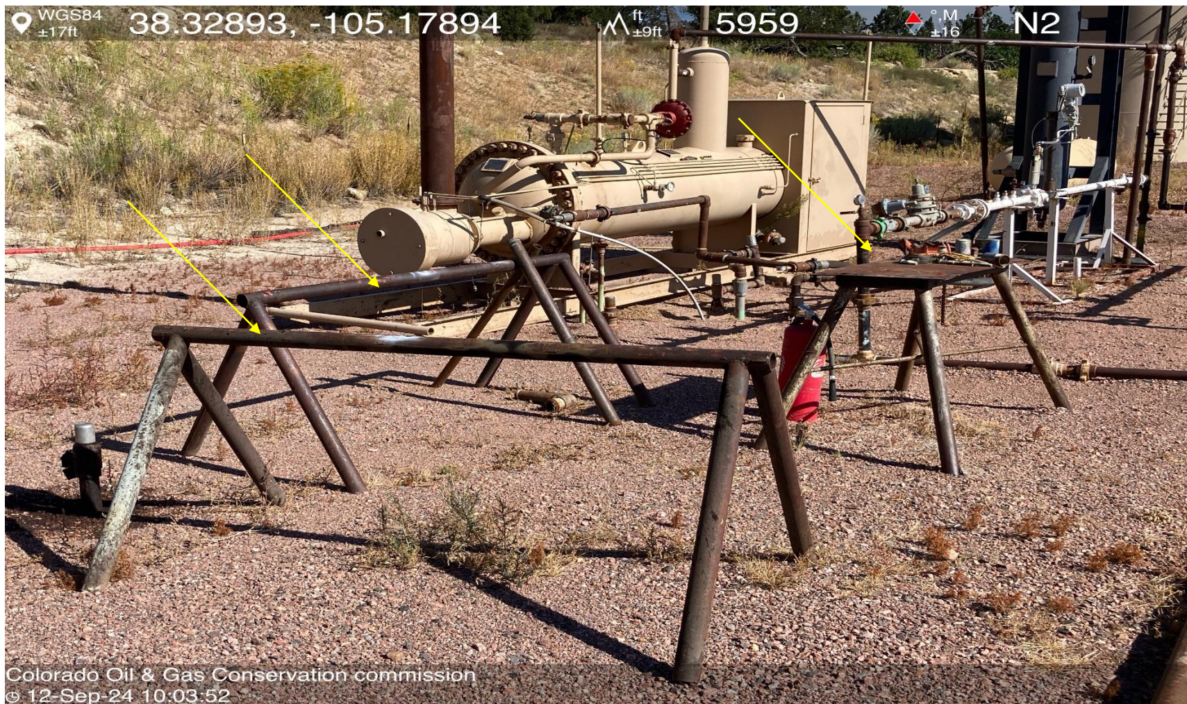
PHOTO 14: UNUSED EQUIPMENT STORED ON LOCATION (WORK BENCH AND SAW HORSES). REMOVE ALL UNUSED EQUIPEMENT FROM LOCATION PER RULE 606. CA DATE 9-18-2024.
