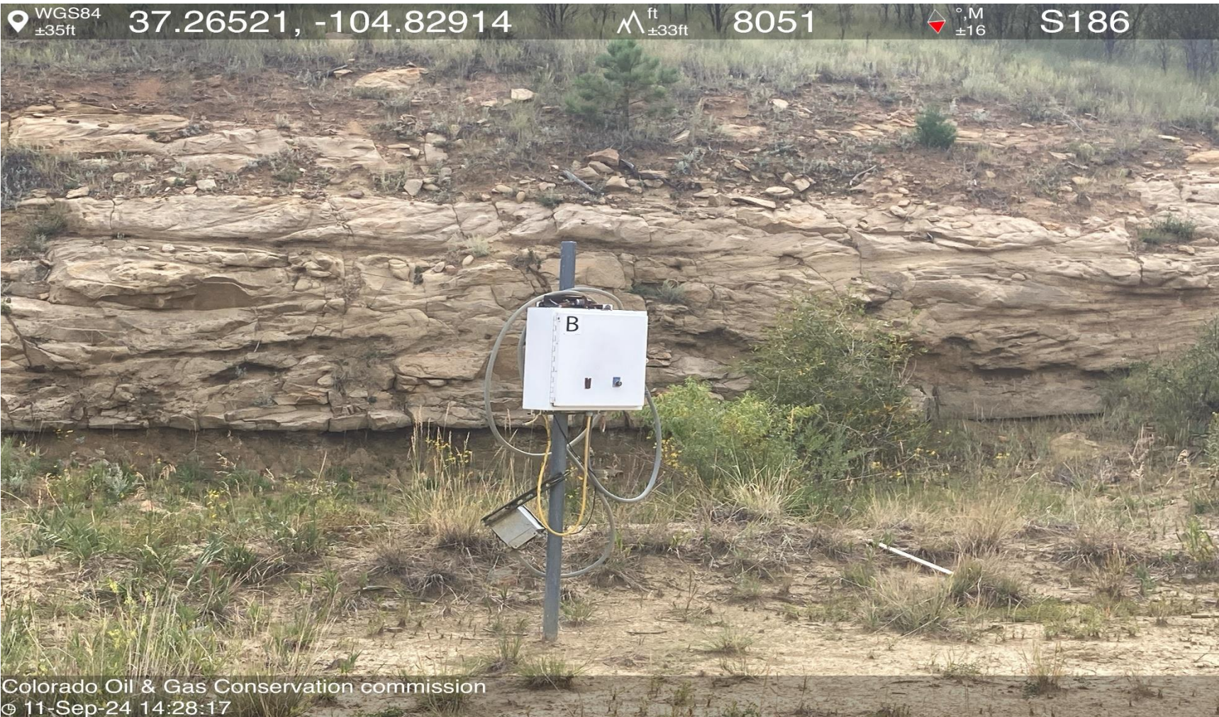
PHOTO 3: UNUSED EQUIPMENT (APPEARS TO BE TELEMETRY EQUIPEMNT). REMOVE UNUSED EQUIPEMENT PER RULE 606. CA DATE 10-12-2024.
