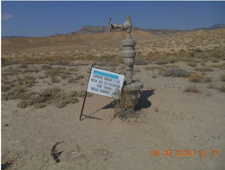
Wellhead with sign. Temporarily abandoned
