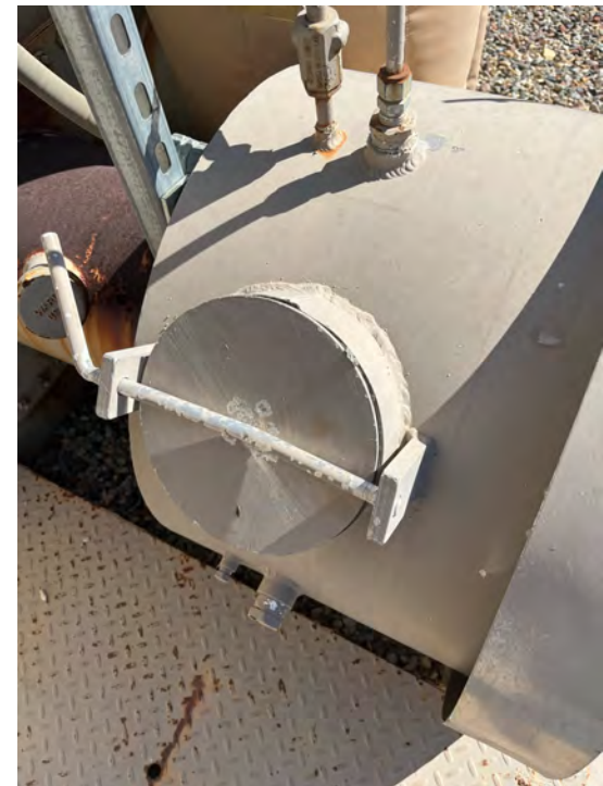
Separator burner is closed - 08/30/2024
