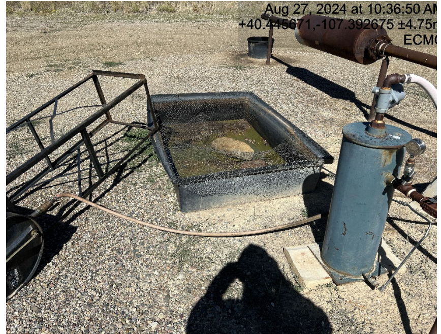
Tank not labeled and not in containment
