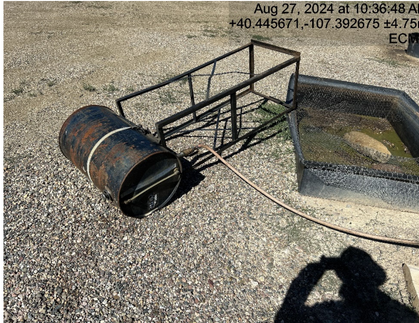
Tank not labeled and not in containment
