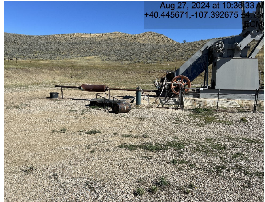
Tank not labeled and not in containment
