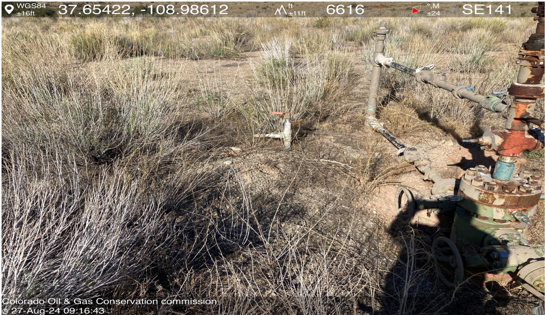
PHOTO 9: UNUSED EQUIPMENT THE WELLHEAD (1" RISER NEAR WELLHEAD). REMOVE UNUSED RISERS PER RULE 606.
