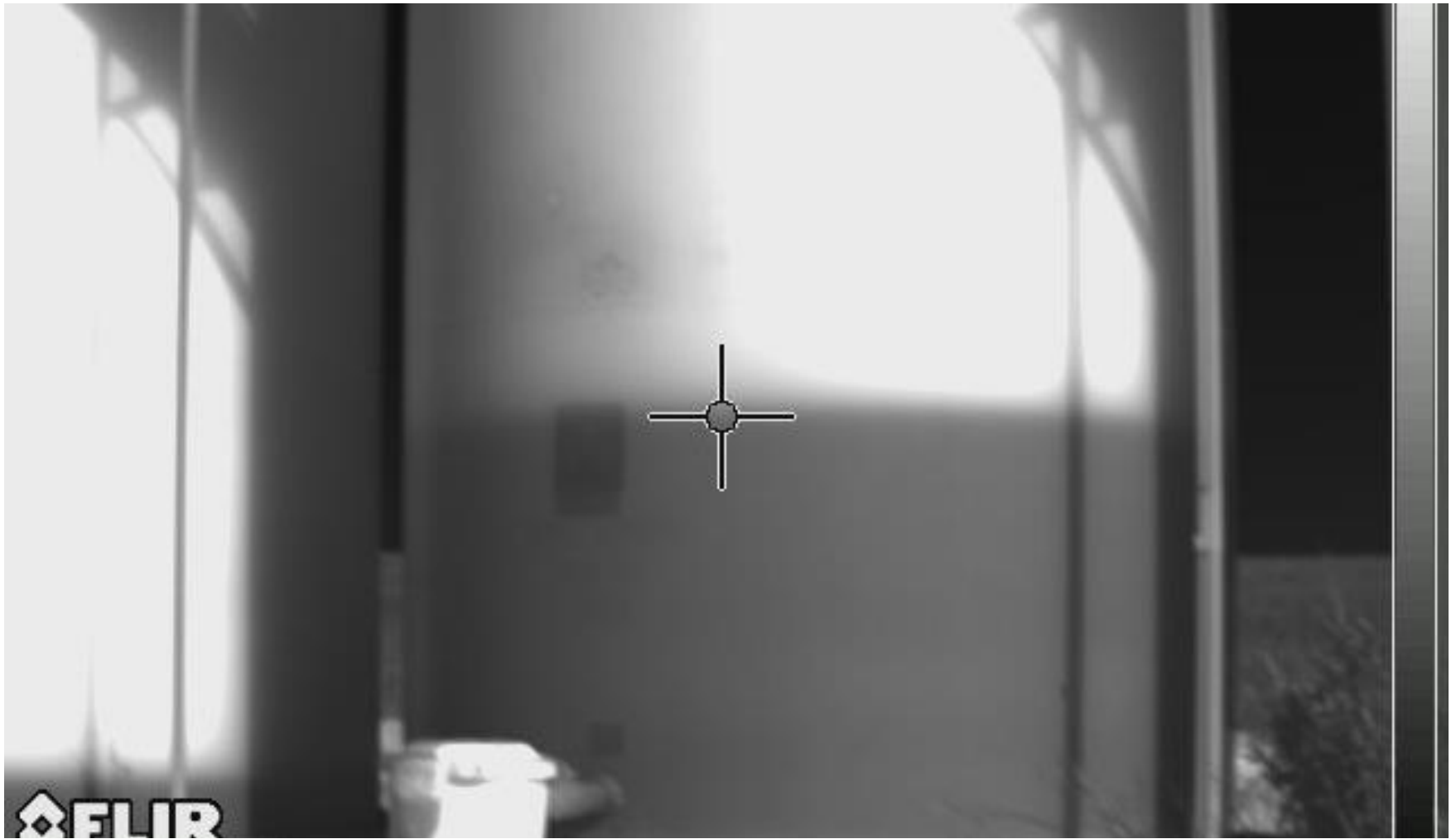
PHOTO 6: FLUID LEVEL IN MIDDLE CRUDE OIL TANK IS APPROX. 7'
