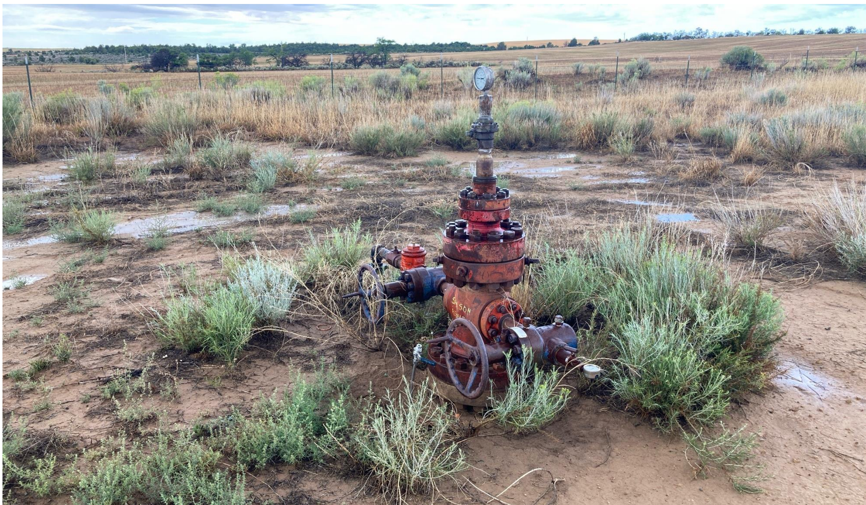
PHOTO 3: WELLHEAD AND EQUIPMENT
