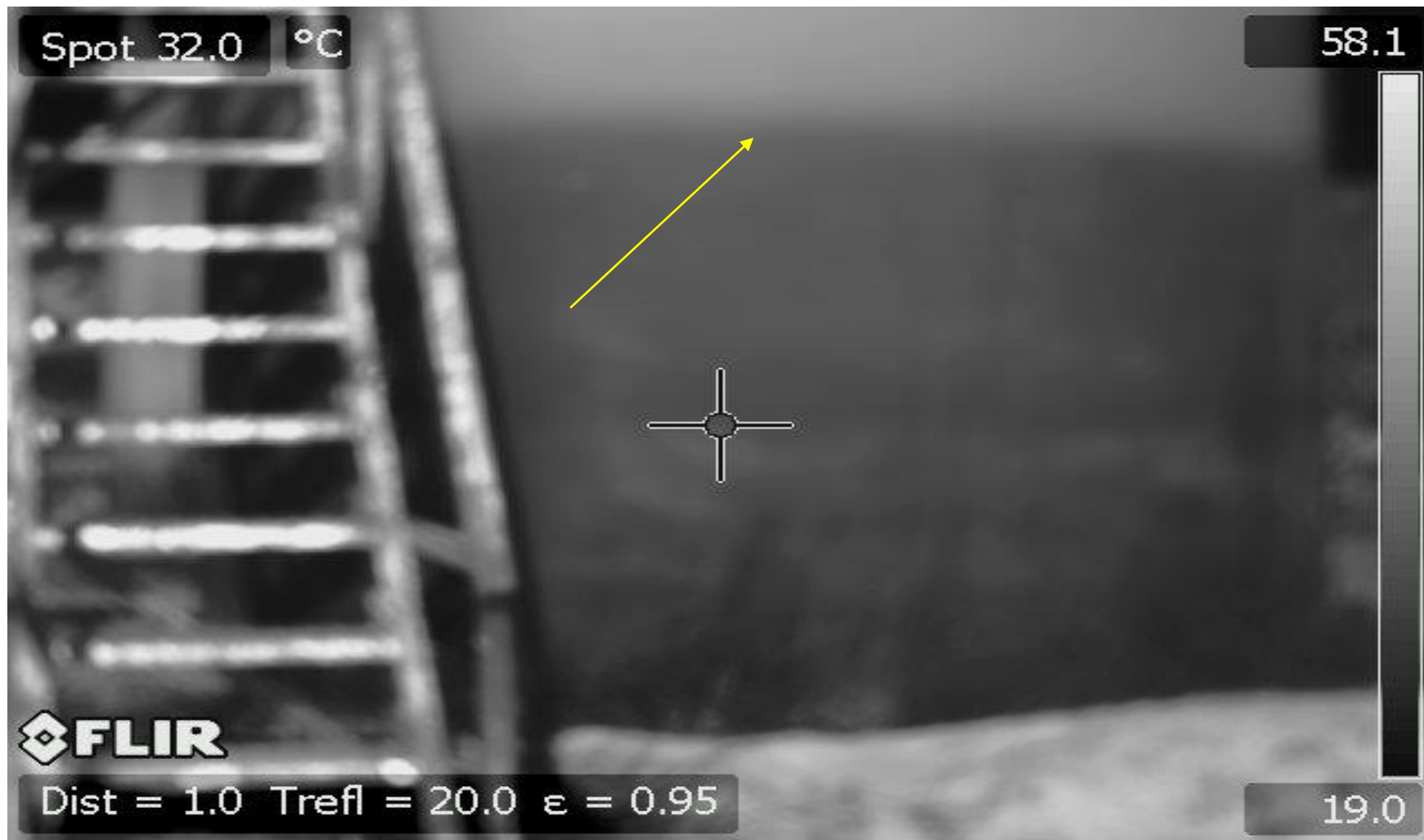
PHOTO 8: FLUID LEVEL INSIDE CRUDE OIL TANK IS APPROX. 6'
