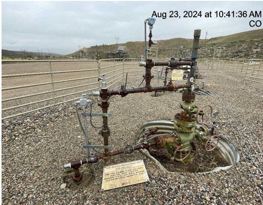
Photo # 6062 Wellhead sign laying on ground & not properly Posted/does not comply with CECMC signage rules
