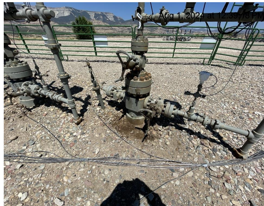
Photo # 4438 Staining near wellhead
