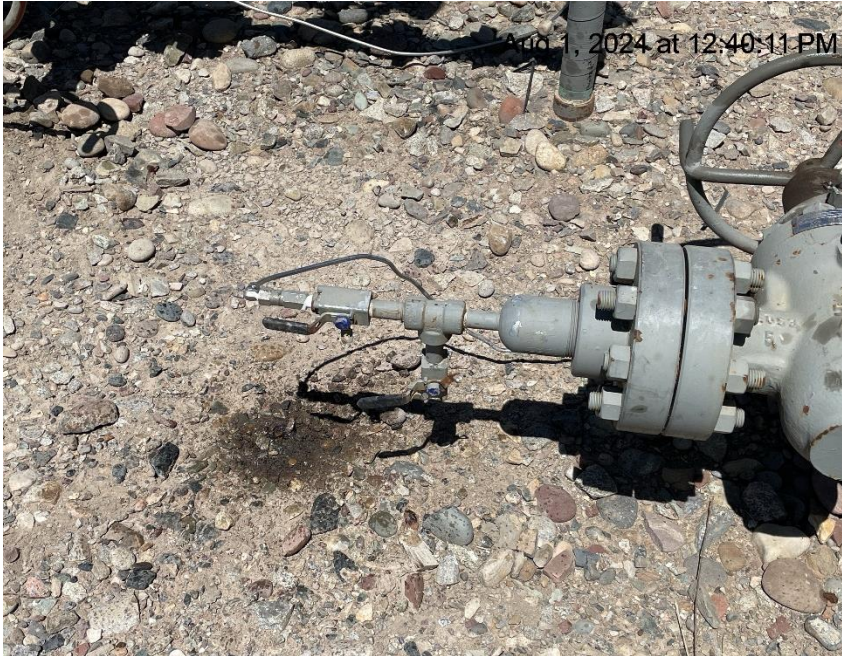
Photo # 4435 Staining near wellhead
