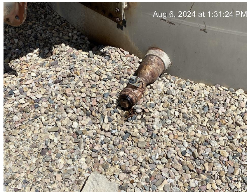
Leaking plug. Stained soil.
