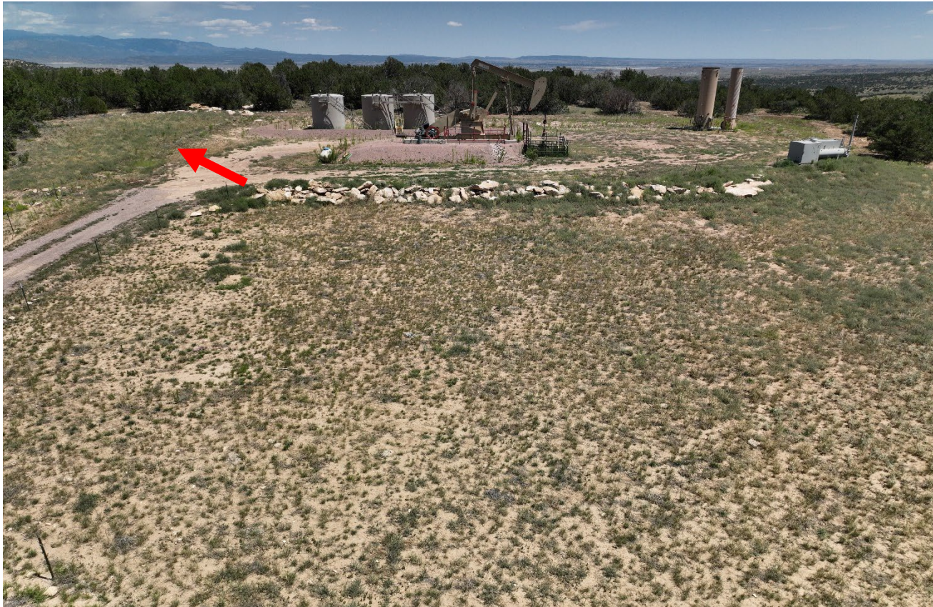
Photo 3. Drone aerial photo facing north toward the wellsite location. The degraded wattles still remain in the upper left at red arrow.
