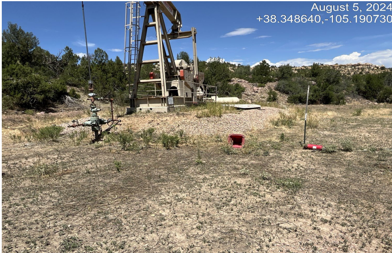
Photo 7. Facing toward the punmpjack. The pumpjack is unused and needs to be removed. The fire extinguisher has fallen over.
