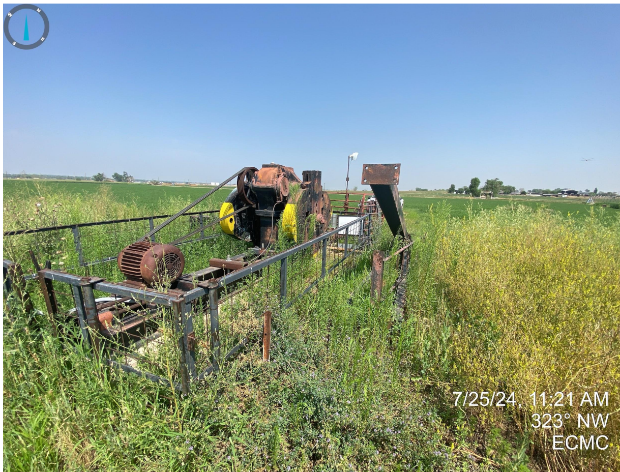
Photo 5. Pump jack is disassembled and unused equipment needs to be removed from the location or returned to service.
