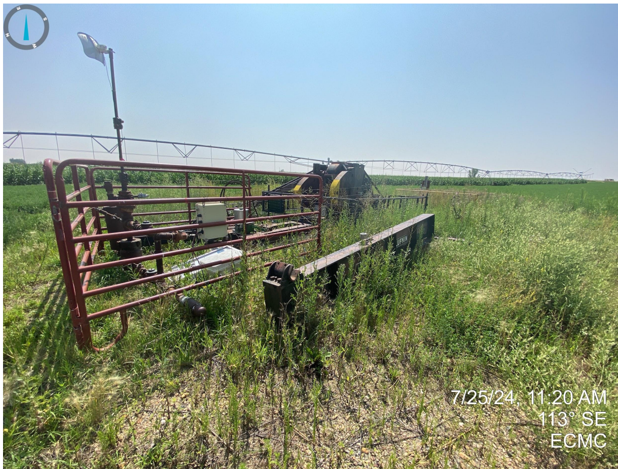
Photo 2. Pump jack is disassembled and unused equipment needs to be removed from the location or returned to service.
