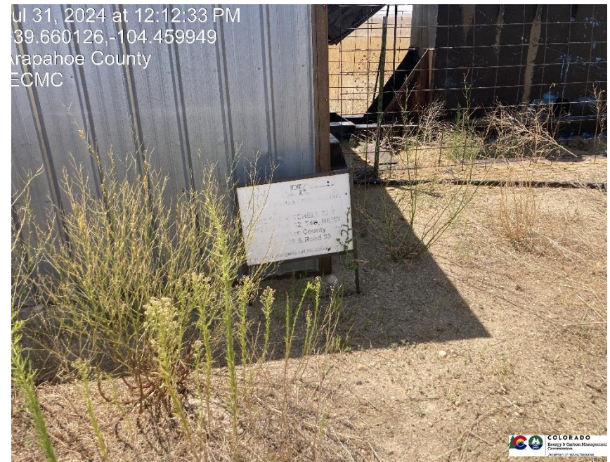
Pic 4 wellhead sign is illegible
