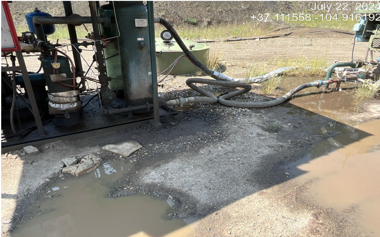
Photo 2. There is oil in the engine skid that has spilled over onto the ground and has mixed with stormwater..
