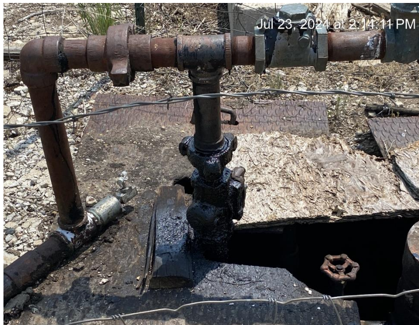
Leak on wellhead
