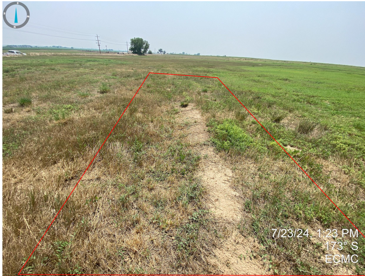
Photo 4. Taken on the western edge of the form tank battery location. Red outline illustrates approximate area of the location that has not been recontoured or graded to reflect adjacent topography.
