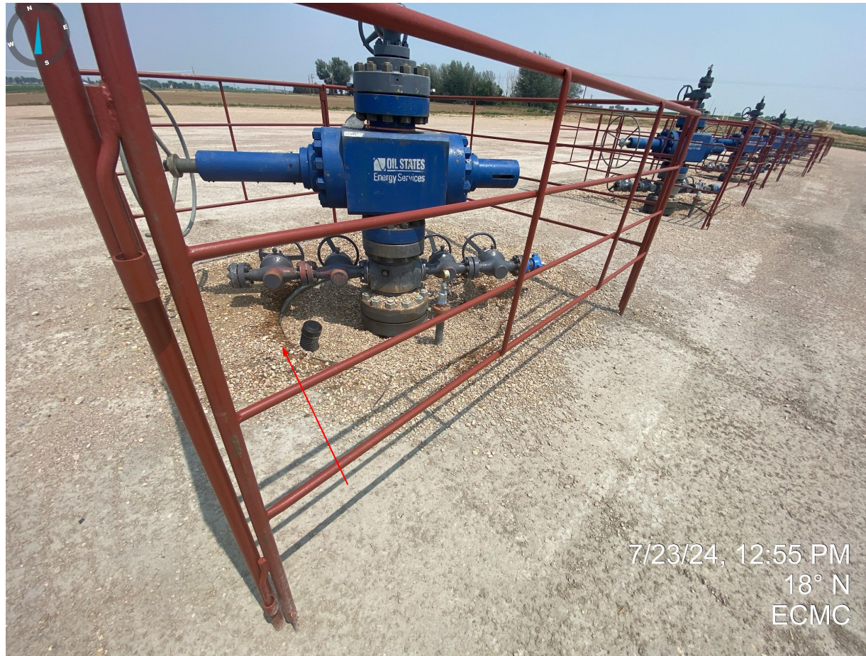
Photo 11. Stained soil observed around conductor at wellhead. Operator shall self inspect all conductors and dispose of stained soils properly.
