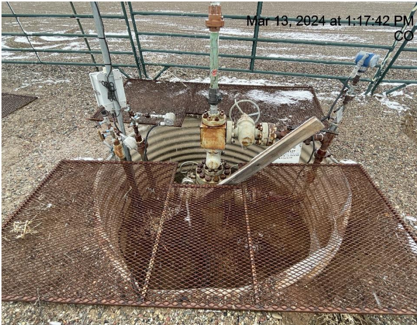
Photo # 9871 From inspection 708903328 conducted on 03/13/2024 Cellar cover not properly installed/wildlife & personnel hazard & wildlife egress not properly installed.
