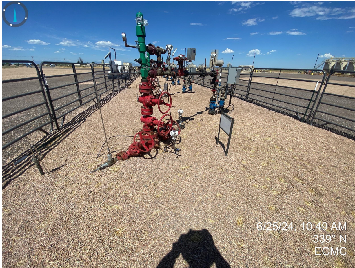
Photo 25. Stained soil around wellheads appears to have been removed and disposed of.
