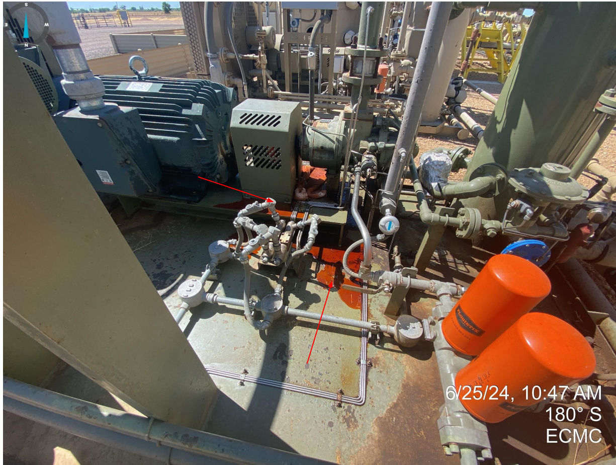
Photo 21. Free fluids observed within compressor skid on west side of location.
