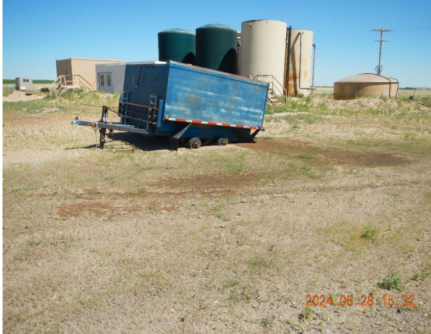
15. Leaking Open Top Tank Trailer. Wet discolored soil area is approximately 30' X 17'.
