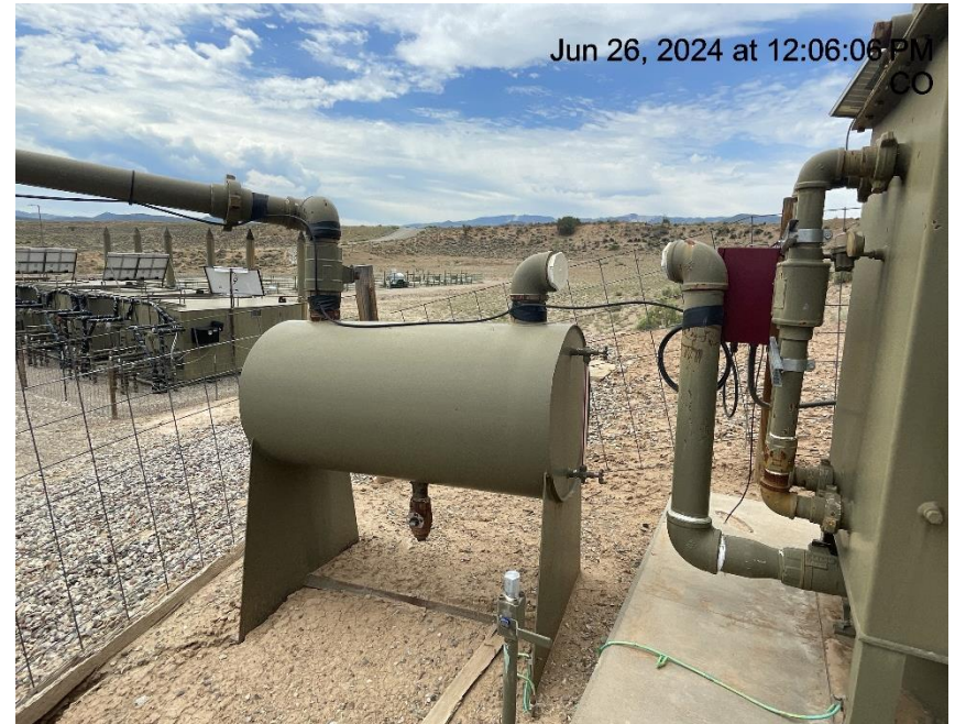
Photo # 1604 Unused equipment – ECD disconnected & not in use
