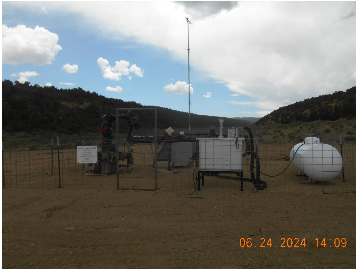
Injection wellhead with line heater and Telemetry
