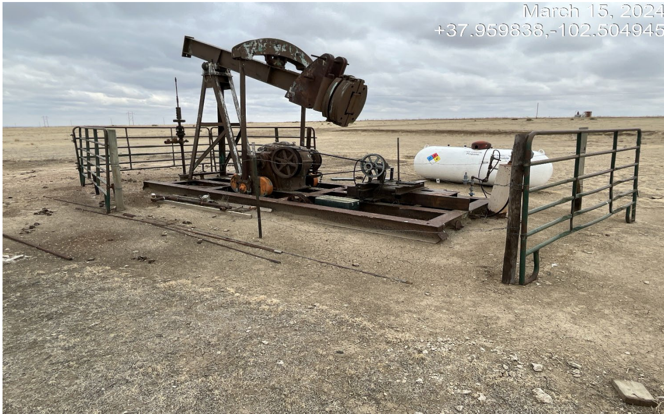
Photo 5. The fence around the pumpjack is insufficient to prevent livestock entry.
