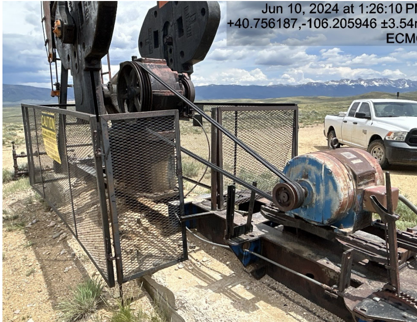
Belt guard is missing
