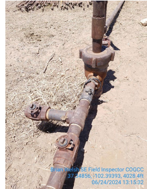
Casing valves at time of inspection are open
