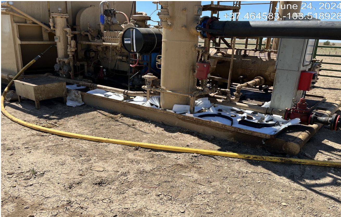
Photo 5. There absorbent cloths used for cleanup. Equipment should be repaired to prevent leaks.
