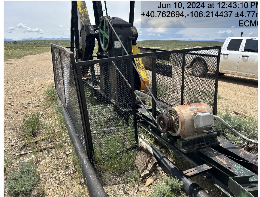
Pump jack guard missing and weeds around equipment
