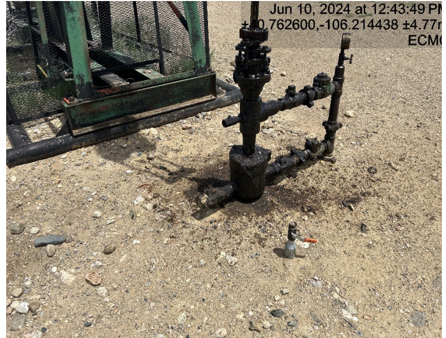
Well head leaking
