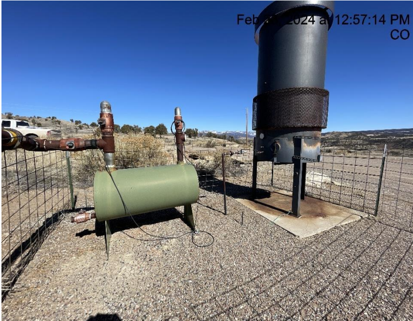
Photo # 7725 From inspection 708903198 conducted on 02/28/2024 Unused Equipment/ECD disconnected
