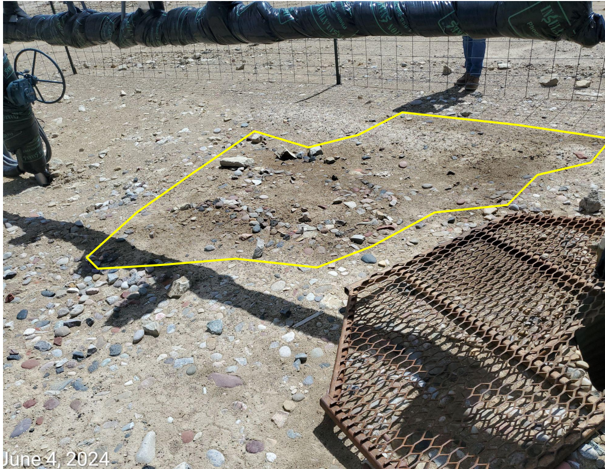
Photo 1: Stained soils around well.
