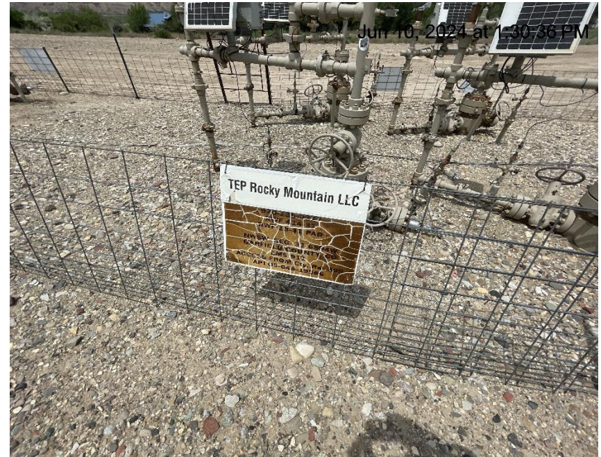
Photo # 222 Wellhead sign weathered & cracking/sign is becoming illegible & does not comply with CECMC rules
