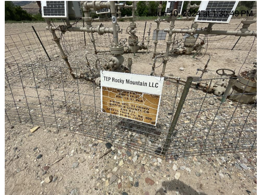
Photo # 224 Wellhead sign weathered & cracking/sign is becoming illegible & does not comply with CECMC rules
