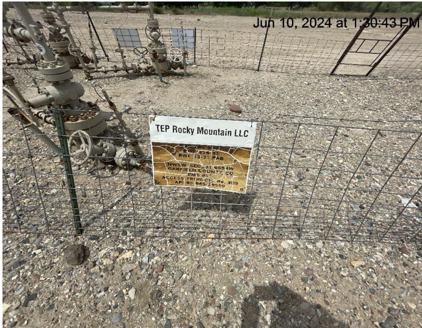
Photo # 223 Wellhead sign weathered & cracking/sign is becoming illegible & does not comply with CECMC rules
