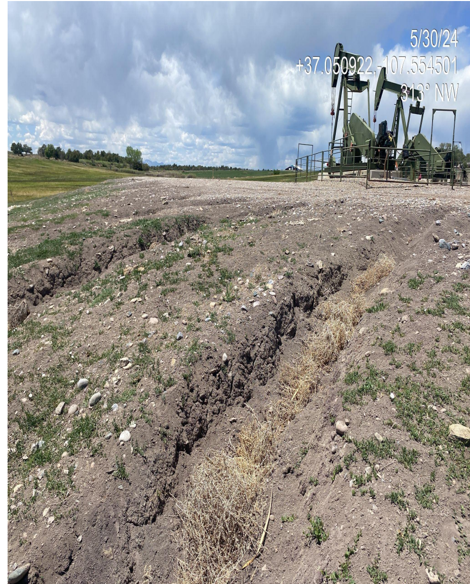
Photo 3. Sever gully erosion observed forming throughout the southern portions of the interim reclamation area, additional stabilization is needed.
