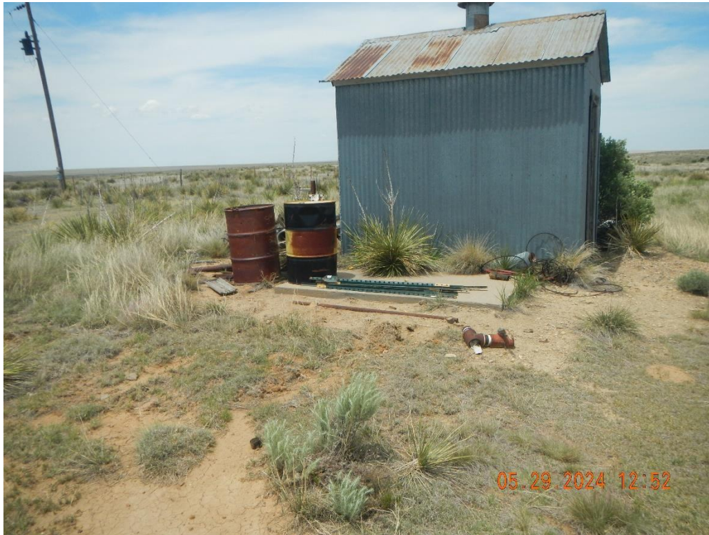
Barrel of Lube without secondary containment.
