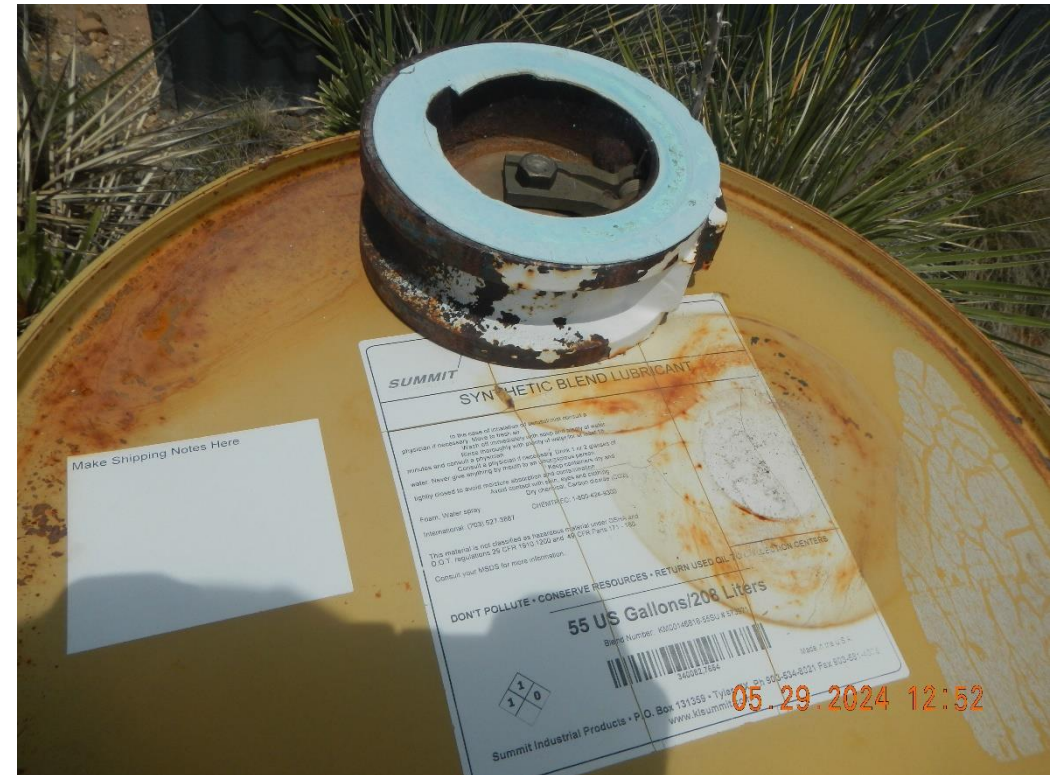
The smaller bung cap is missing from barrel and covered with a pressure release valve.
