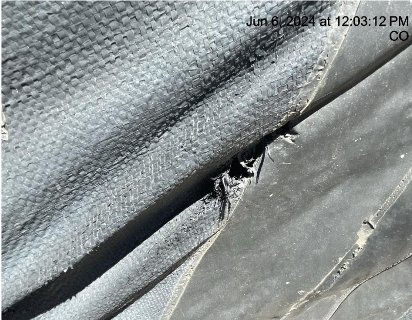
Photo # 9973 Hole in liner/liner needs maintenance
