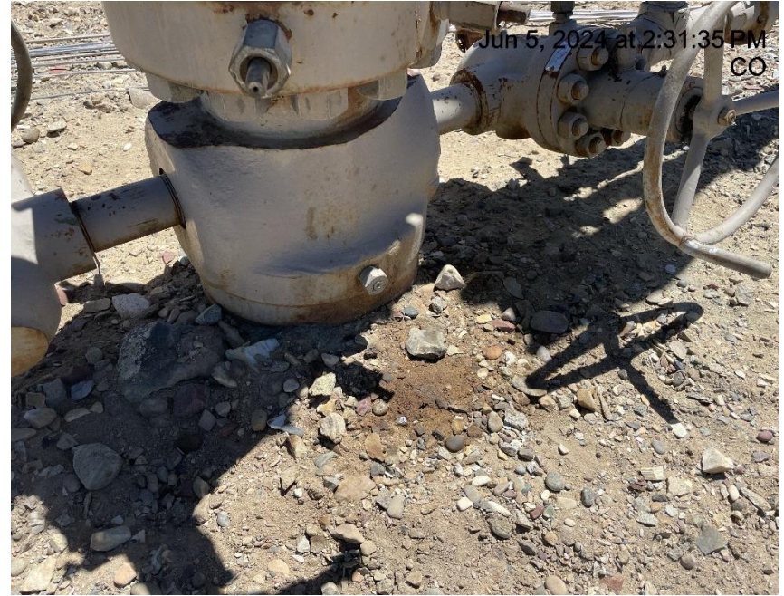
Photo # 9795 Staining near wellhead
