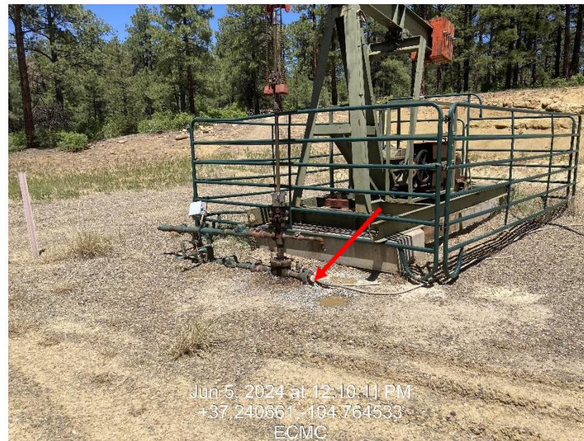
Photo 4 – White staining around wellhead
